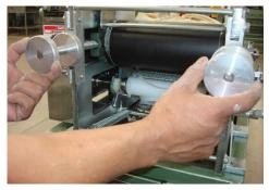
Adjust the tortilla thickness by turning the adjustment knobs (clockwise to make the tortilla thinner, and counterclockwise to make it thicker).
