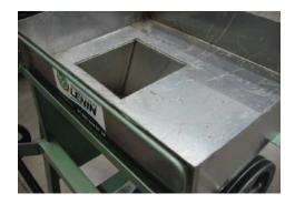
Turn on equipment and place the product in the 2 hopper to start grinding.
