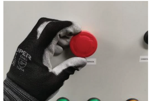
B Unlock emergency stop
