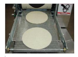
Check the cut and thickness of the tortilla.
