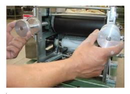
Adjust tortilla thickness by turning the adjustment knobs (clockwise thins the tortilla, counterclockwise thickens the tortilla)
