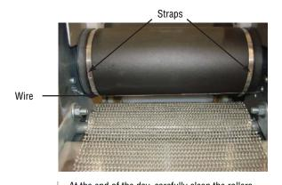
At the end of the day, carefully clean the rollers, especially the straps and wire, trying not to leave mass residues that could cause the wire to break on the next use.
